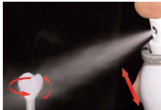
Spray the IPS e.max CAD Crystall./Glaze Spray directly on the unfired IPS e.max CAD Crystall./Shades and Stains. Spray the restoration from all sides while simultaneously rotating it.
