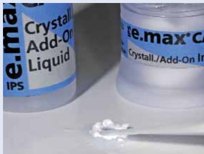
Mixing of IPS e.max CAD Crystall./Add-On with IPS e.max Crystall./Add-On Liquid to a ductile consistency.
