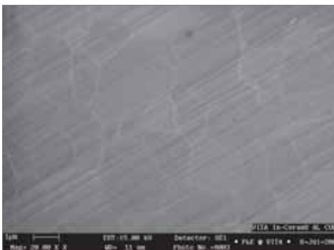
Fig.2: SEM-photo of the microstructure of a sintered VITA In-Ceram AL (Magnification x 20,000).
